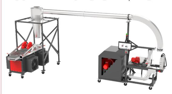
**ECON** Vibration system offers superior cooling performance by gently moving your product forward to the discharge.
