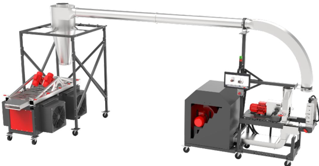
**ECON** Vibration system offers superior cooling performance by gently moving your product forward to the discharge.
